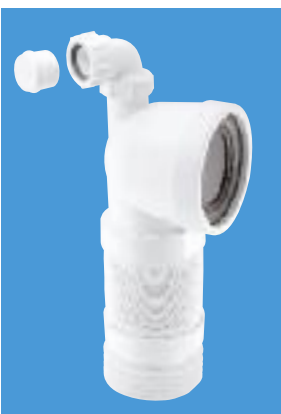
97-107mm Inlet 4"/110mm Outlet 1 1/4" Universal Vent Boss
