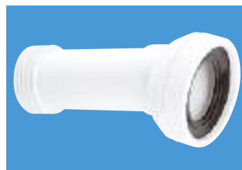
14° Angle Adjustable Length 97-107mm Inlet 3½"/90mm Outlet
