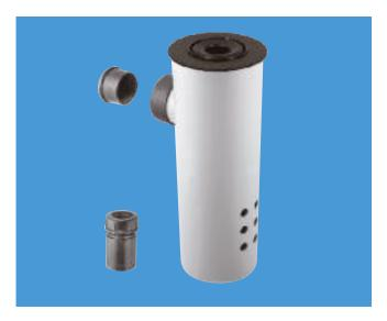
110mm x 300mm x  $1\frac{1}{4}$ "/ $1\frac{1}{2}$ " Pipe top and side Inlet Connections to receive discharge from a condensing boiler. 19/23mm x  $1\frac{1}{4}$ " fitting provided to increase size of discharge pipe before it passes through the external wall
