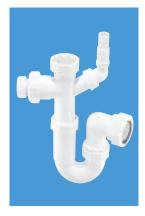
1½" x 75mm Water Seal Tubular Swivel Sink Trap with adjustable inlet, nozzle for discharge hose of domestic appliance and connection for 19/23mm pipe. Supplied with blanking cap
