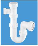
1½" x 75mm Water Seal Tubular Swivel Sink Trap with adjustable inlet and connection for 19/23mm pipe. Supplied with blanking cap
