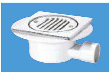
150mm Square Polished Stainless Steel Tile with removable Grid and Securing Screws 1½" BS EN 1329-1:2000 solvent weld horizontal outlet. Overall height 75mm
